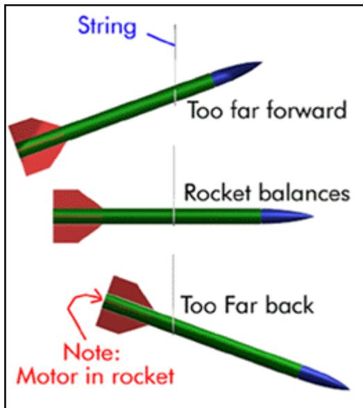
Put a motor in your rocket and tie a string around the middle. Move the string until your rocket balances. The point at which it balances is your Center of Gravity.
