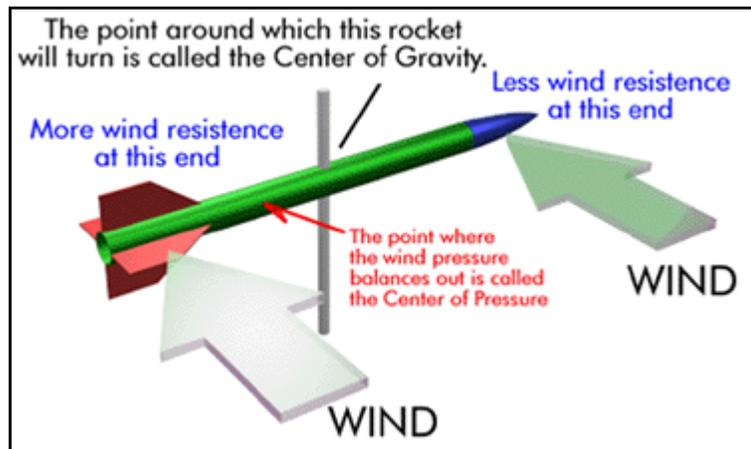
Pretty simple? Don't worry about the Center of Gravity and Pressure just yet. We're getting to that. The idea here is that it is the pressure of air flowing over the rocket which pushes it around like a weather-vane. My example is rather two dimensional. Real rockets are affected like this from all directions.
