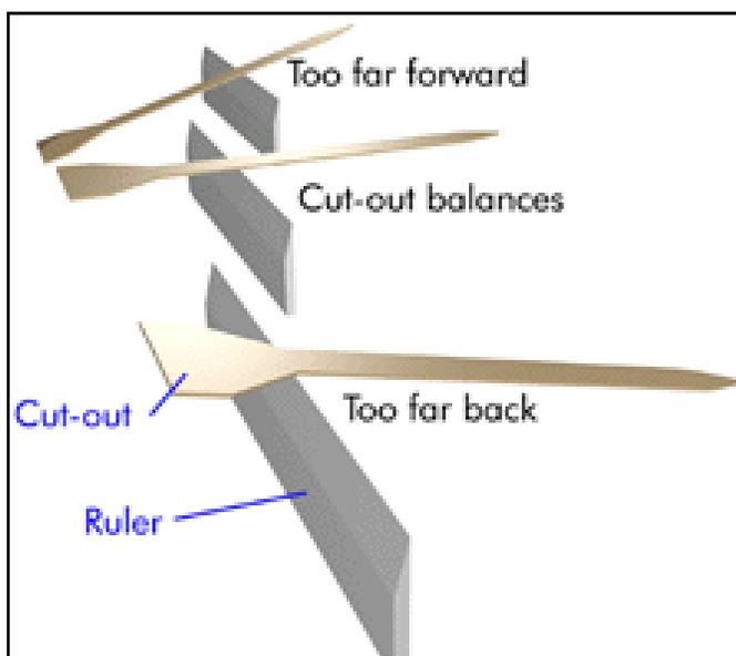
**Step 2:** Balance the cut-out on the edge of a ruler. Mark where it balances. This spot marks the Center of Pressure of your rocket.
