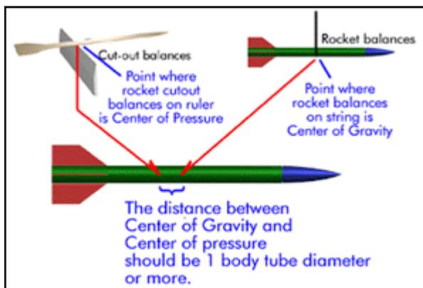
Now you have the two most important things you need to determine your rockets stability. The CG is the point around which your rocket turns, like the axis on a weathervane. The CP is where the cumulative pressure of wind appears to be pushing against. If your CG is in front of your CP, your rocket is stable. Here's how to check further for rocket stability.
