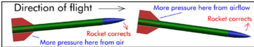
The idea is to make a rocket which will use air pressure to correct its own flight. As the rocket flies upwards, it will try
