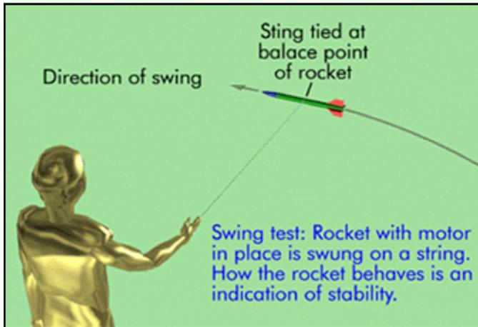
The swing test is a basic test to give you a rough idea how your rocket will fly.
