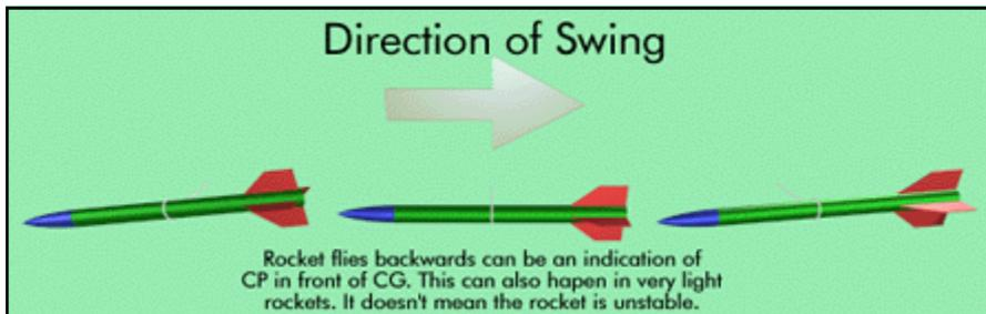
Sometimes your rocket flies backwards. I have had this happen when a rocket is very small or light. The motor is so heavy in comparison, that the Center of Gravity is very near the Center of
