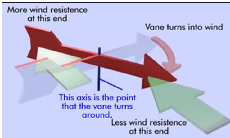
The principle of air pressure blowing against an object and causing it to turn is well demonstrated by a weathervane.
