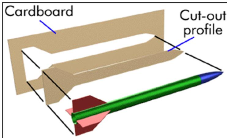
**Step 1:** Cut out a profile of your rocket in cardboard. It doesn't have to be the same size, but it does need to be accurate in shape and scale.
