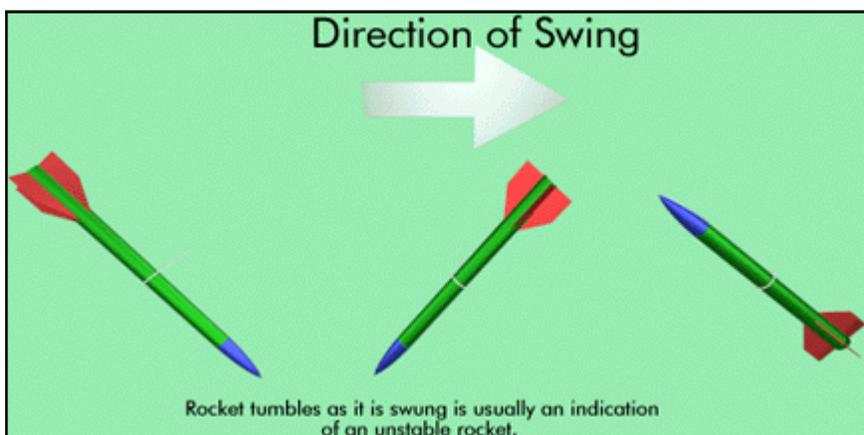
Sometimes a rocket will just cartwheel as you swing it. It is usually a sign that the CP and CG are too close together. Try adding a little weight to the nose, and see if your rocket straightens out.
