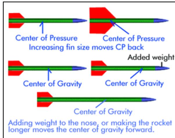
Well, those are the basic ideas when trying to check the stability of a model rocket. I suggest checking the CP and CG on rockets that you know are good flyers, and then trying to match that on your own scratch built versions. After awhile, you will be able to almost see where the CP on a rocket will be, and you will only need to do a swing test on unusual shaped rockets.
